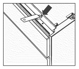
Insert the tab of each bracket into the guide holes on top.
